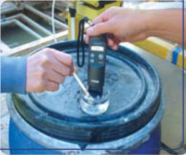
Treated waste water is tested prior to recycling 經處理的污水須通過測試才可循環再用
